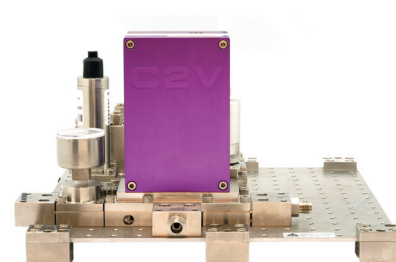
C2V-200 micro GC on NeSSI platform
